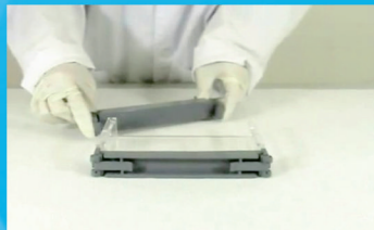
Dams-claw专利灌胶模具，简单拆装，容易清洗
