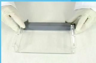
Dams-claw专利灌胶模具，简单拆装，容易清洗
