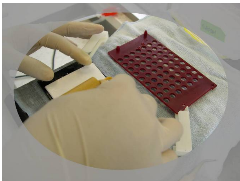
Figure 6: Slightly remove the air bubbles by the roller.
