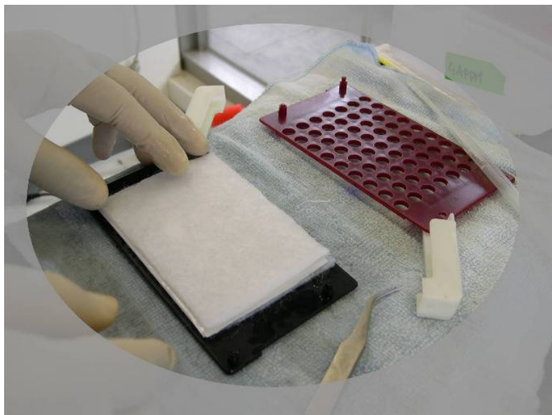
Figure 8: Put the other wet sponge. All the components have to be placed centre within the two sponges. This assembly is also called "sandwich".
